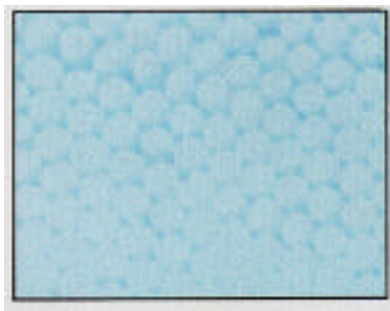
A microscopic view of the silica spheres in opal - Photo courtesy of Office of Mineral Resources, PIRSA.
